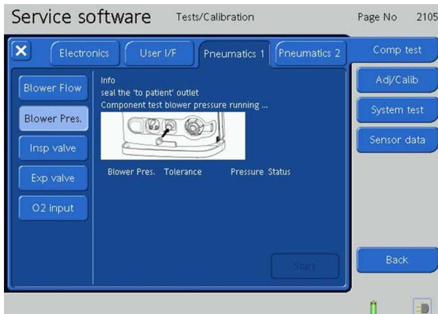
Figure 9-111. The Blower Pressure Tests, Step 2
