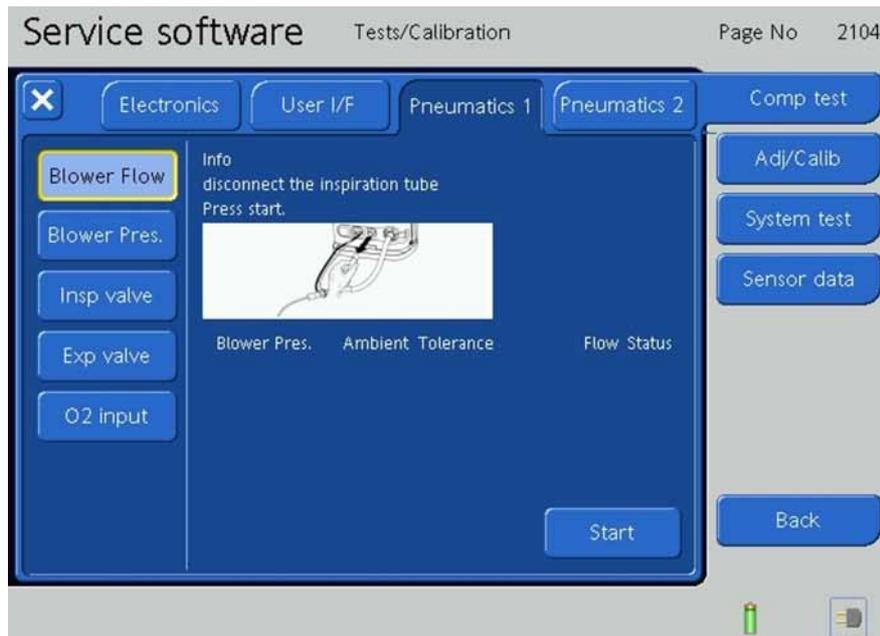
Figure 9-107. The Blower Flow Tests, Step 1
