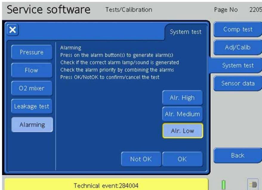
Figure 9-167. The Alarming Screen Tests, Step 4
