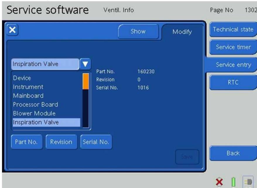
Figure 9-17. The Service Entry Modify Tab Screen, Step 3
