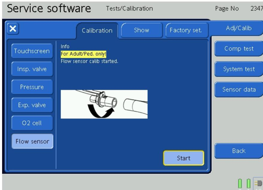
Figure 9-61. Flow Sensor Calibration
