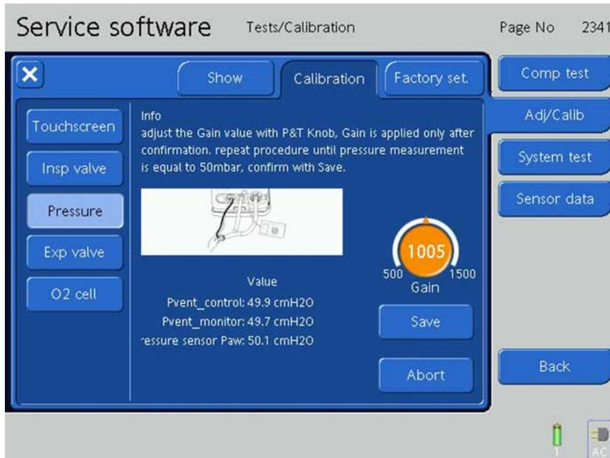
Figure 9-47. The Pressure Adjustment / Calibration, Step 2
