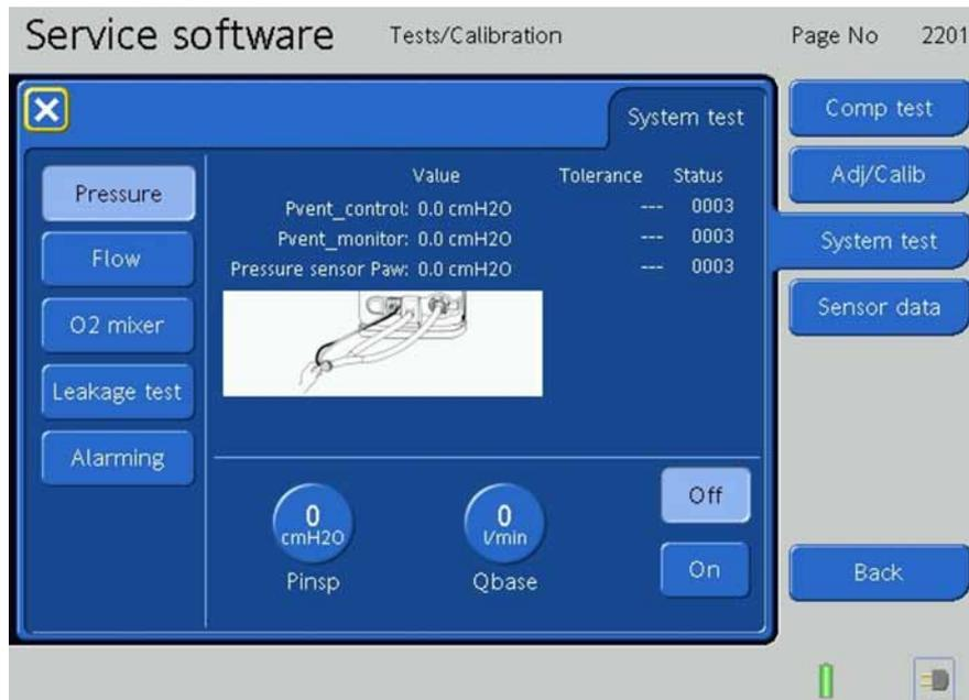
4. Set PInsp to **5, 25 and 50cmH2O**. Press the PInsp Button with the P&T Control Knob. Press the P&T Control Knob and rotate the setting to these values. Press the P&T Control Knob to activate the setting.
