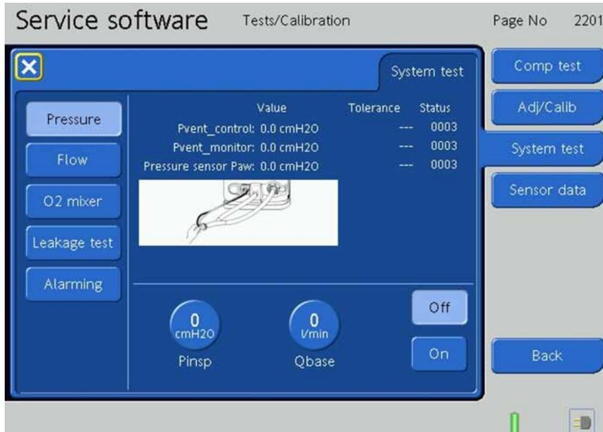
Figure 9-156. The Pressure System Tests, Step 1
