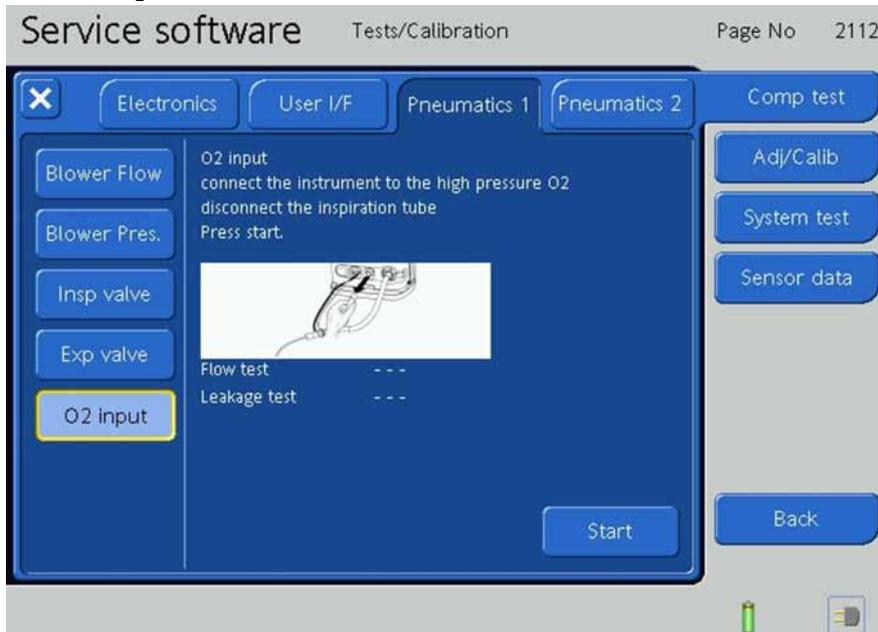
Figure 9-123. The O<sub>2</sub> Input Tests, Step 1
