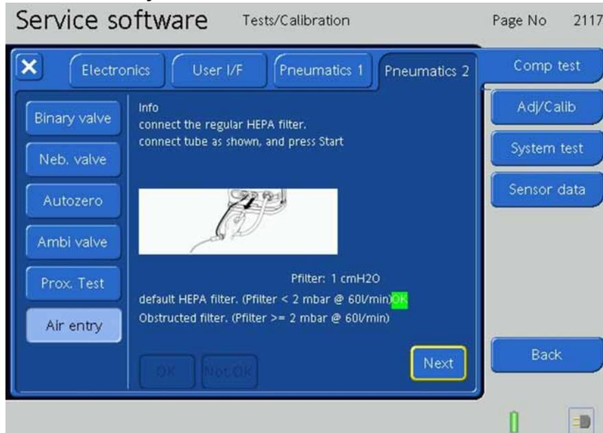
Figure 9-153. The Air entry Tests, Step 1
