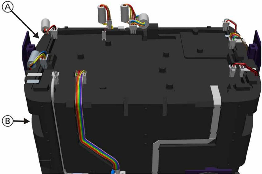
**Figure 11-74. Top Foam Section and Mainboard Assembly, Step 1**
