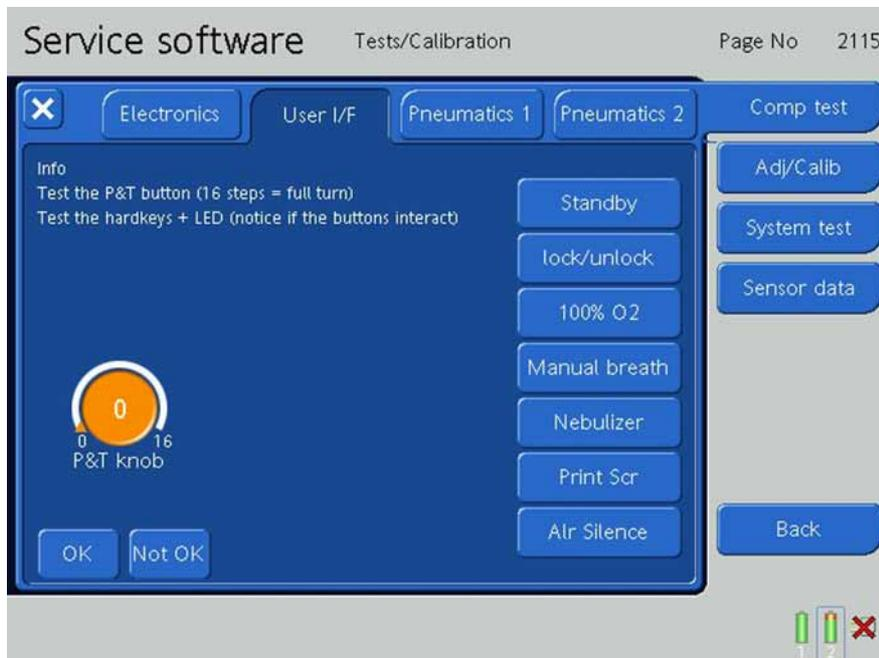
**Figure 9-103. The User Interface Tests, Step 1**
