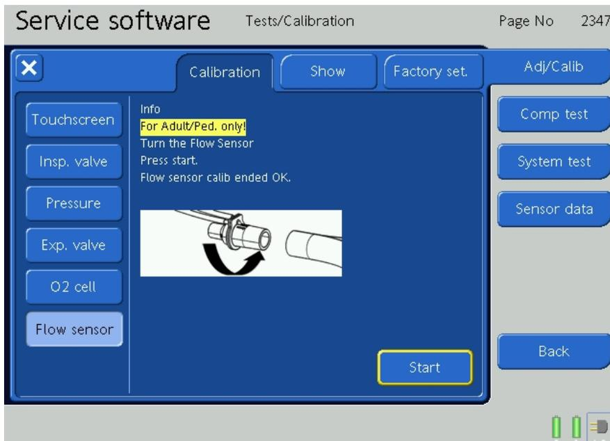
Figure 9-64. Flow Sensor Calibration
