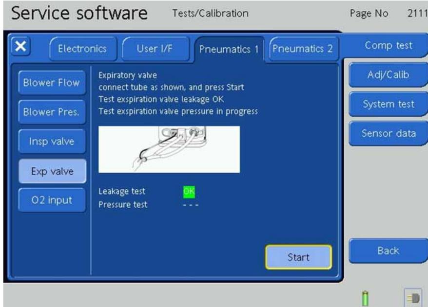
Figure 9-120. The Expiratory Valve Tests, Step 4
