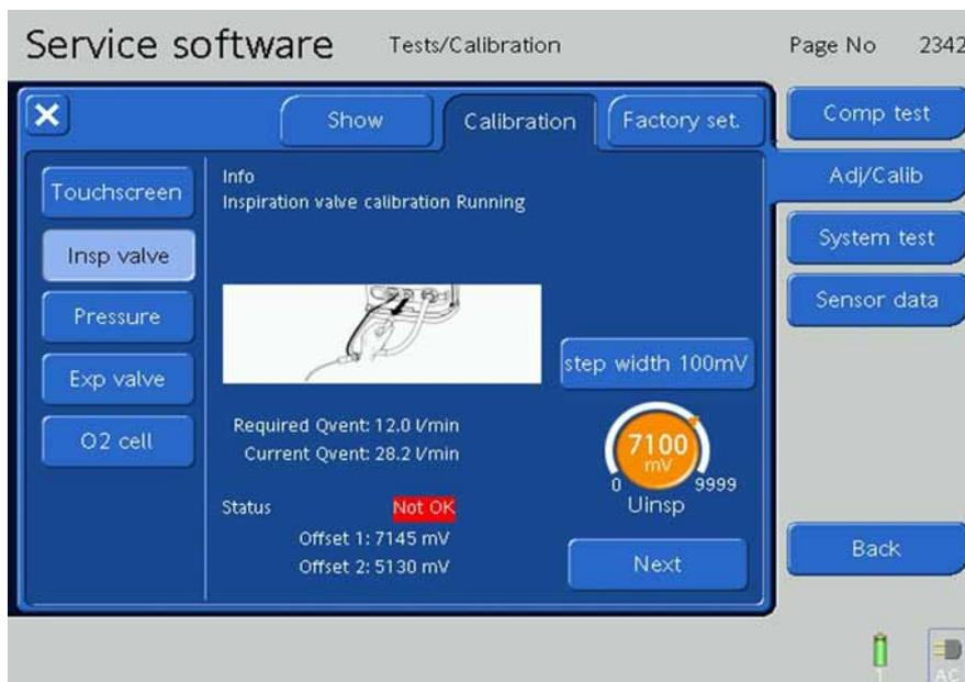
**Figure 9-43. The Inspiratory Valve Adjustment / Calibration**
