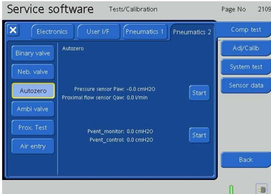
Figure 9-136. The Autozero Valves Tests, Step 1
