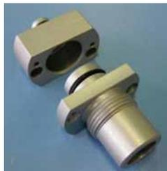
**Figure E-9. NIST connector with mounting adaptor**
